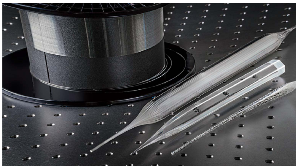
Fig. 1: Spooled fiber and three different fiber preforms from the fiber drawing process.
