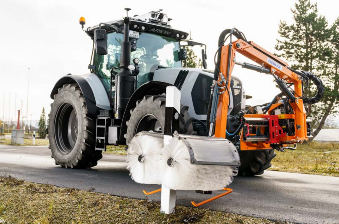
Reduces employee workload and increases safety: automated delineator post cleaning.
