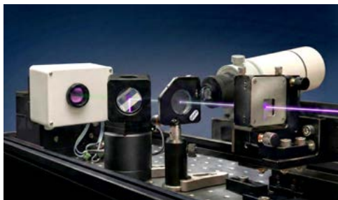
Laboratory setup for Quantum Ghost Imaging.
